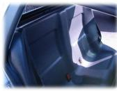
The rear seats are made of composite plastic, as is the rear floor well with built in drainage points - essentially enabling cleaning to take place that is thorough and hygienic.
