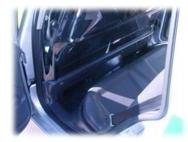
The EVO rear stowage framework also acts as a mesh bulkhead to secure the detainee, but is hinged to enable the detainee to be released in the event of an incident that compromises access via the rear side doors.
