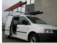
This truly unique ladder management system from the USA is engineered to provide the user with a safe mechanism for the loading and unloading of ladders. The system is activated by a swinging arm (that when in the travel position acts as a secure load lock) that is easy to use, the load frame lifts and delivers the load to the side of the vehicle. Nearside and Offside solutions are available, <u>and they are engineered differently.</u>
